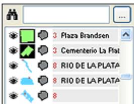
**Object Inspector** box at right side of the main Mawpel window displays information about respective map objects and simplifies the object manipulations. It also allows to select one or several objects in the work space.
