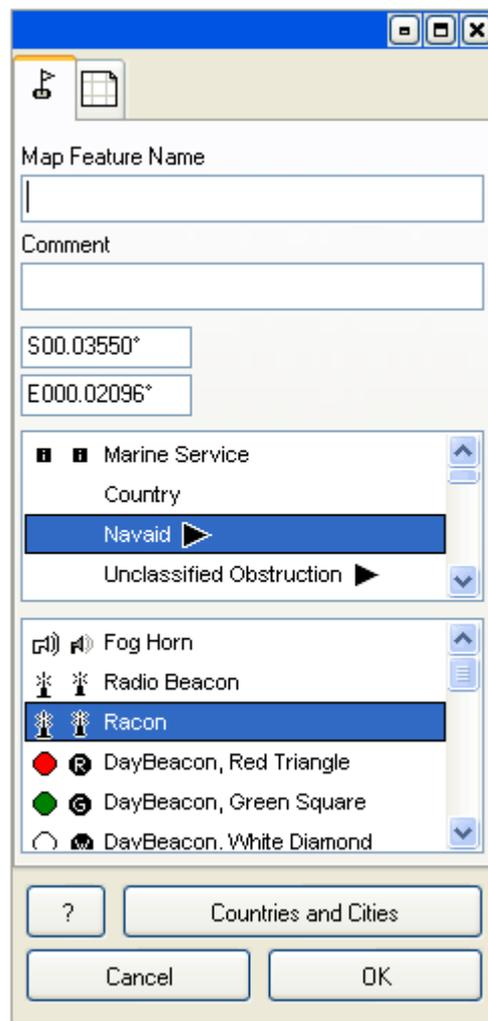
Duplicate the Racon symbol and place it on the proper spot on the map. This simple example map is finished now. To check how it will look like in the color or monochrome display GPS click on **'Color'** or **'Grey Scale'** tabs in the bottom left corner of the Mapwel. You can switch between the tabs anytime during the map creation.
