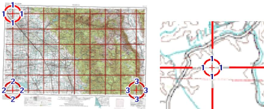
Left: image with calibration points positioned on intersections of grid lines. Right: detail.
