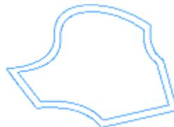
**Shrink Objects** reduces size of selected objects by offsetting the object contours. Shrink Objects command does not provide the same result as normal size reduction.
