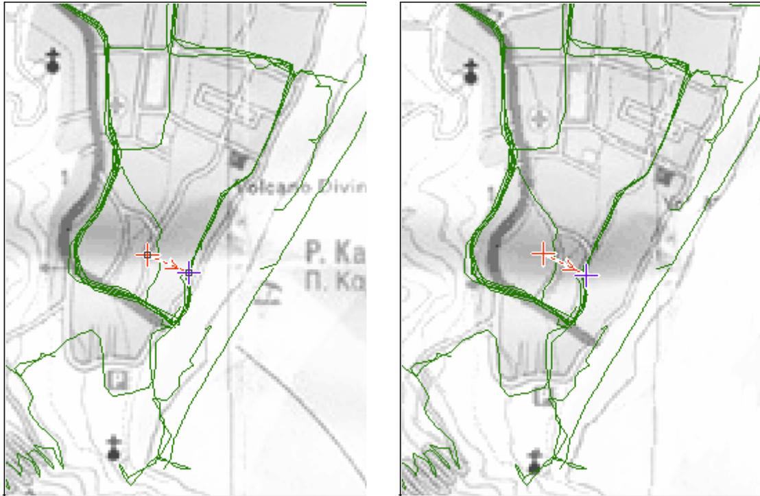
Fig. 3. Image with single pair of calibration points before calibration (left) and after calibration (right).
