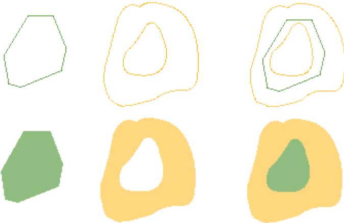
The green object is the area that is displayed behind others (park, in this example). We need to make an opening in the surrounding land to make park visible (it shows through the opening). Notice that the two areas overlap. This is very important, because GPS could display tiny gap between the two areas, otherwise.
