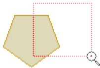
Opening can be used only after Area or previous Opening object. It does not appear in Object Inspector window as a separate object and cannot be selected directly on the Work Area. To select the Opening object for transformation, use the Part Inspector window.
